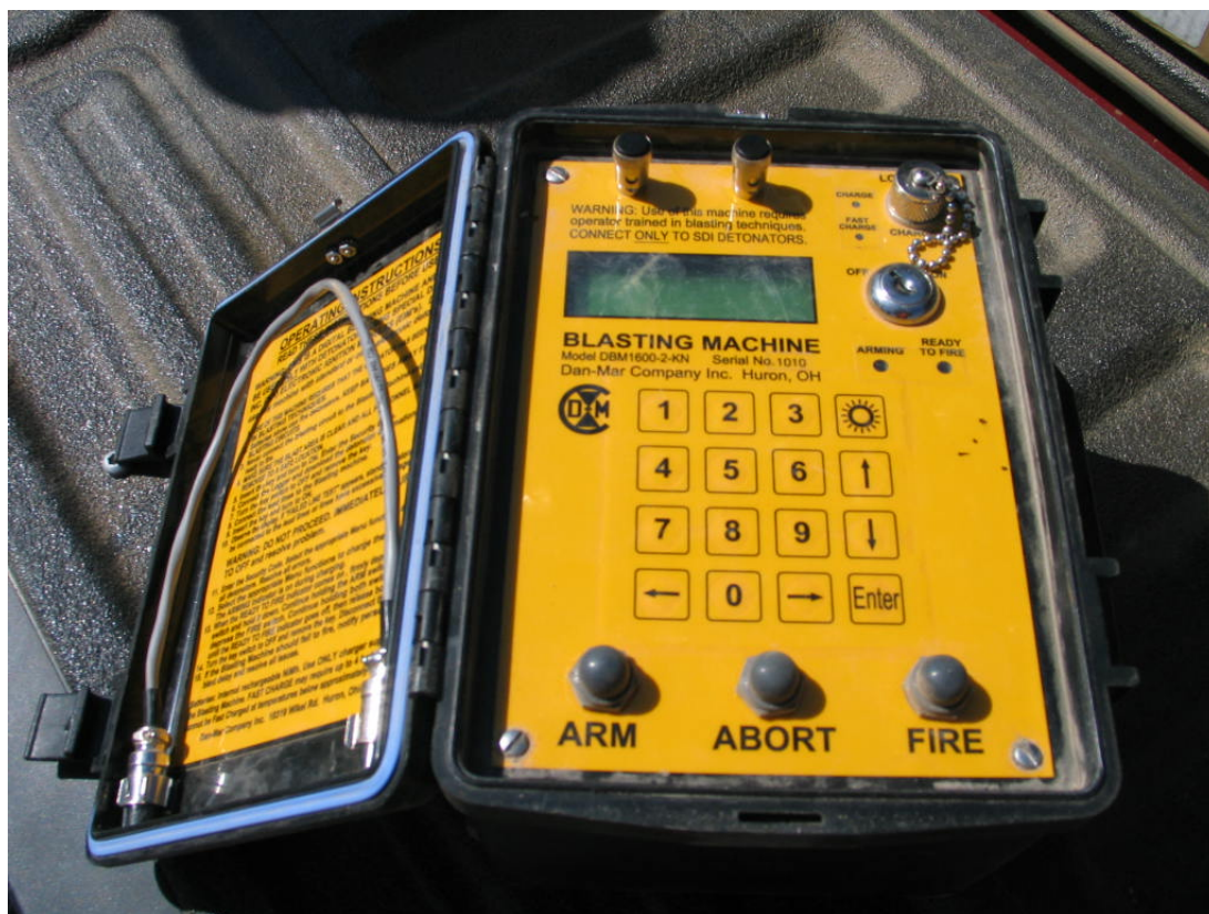
Figure 10 - Dan-Mar Blasting Machine
